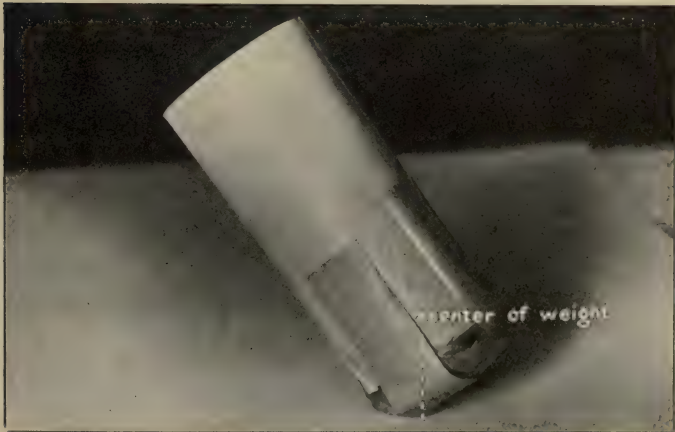
FIG. 16. But in this one the center of weight is so low that it is over the base, no matter what position the cylinder is in.
